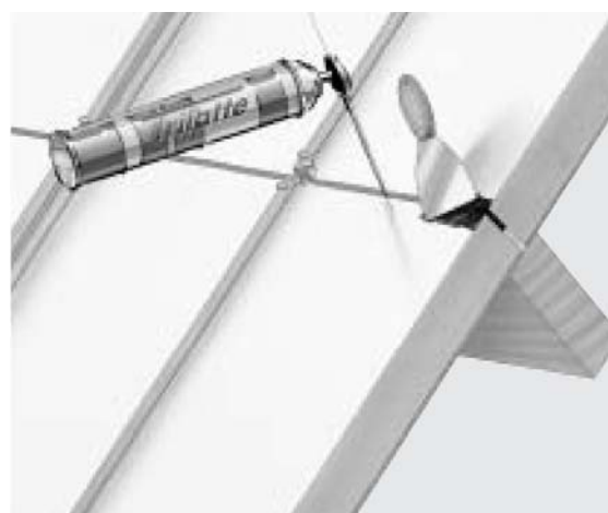
Figure 5 - moussage des joints transversaux
